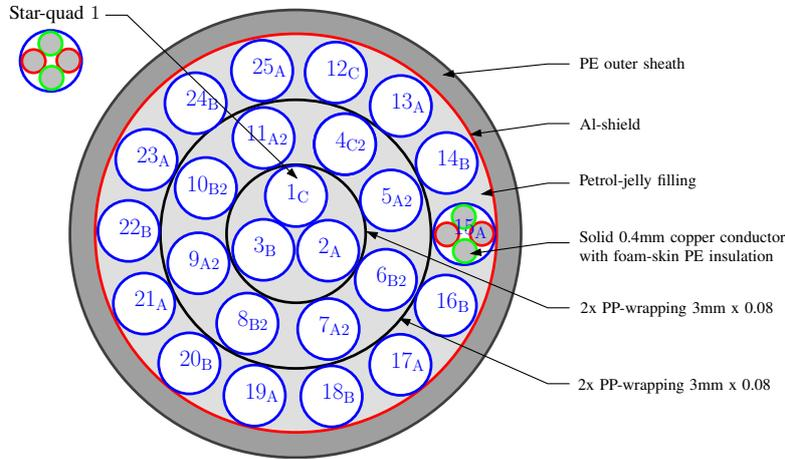
Figure 1: Cable structure
