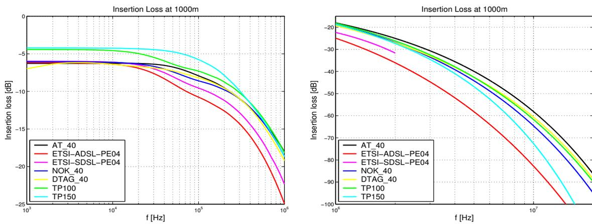
Figure 7: Zooming in on the insertion loss curves for various 0.4mm cable models
