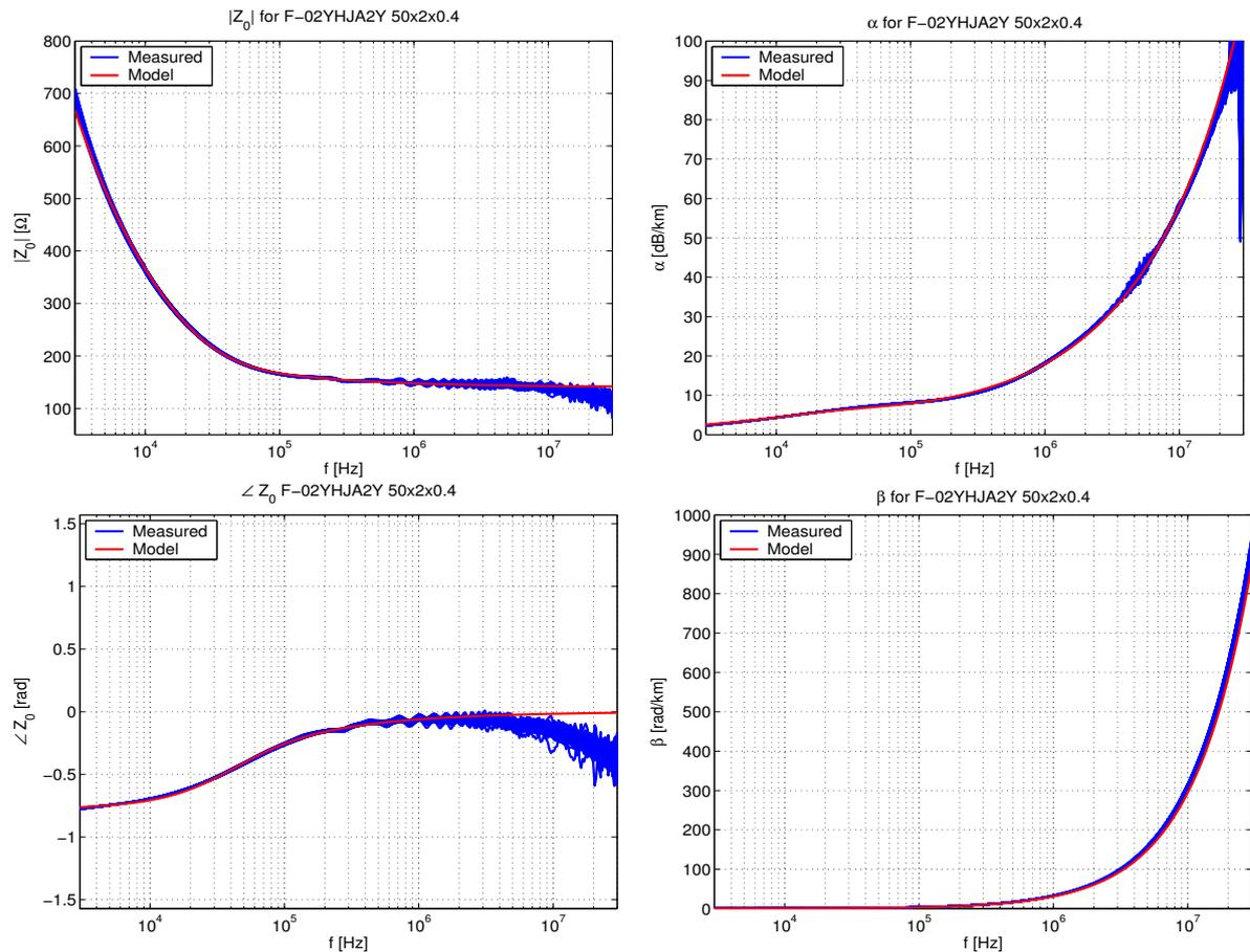
Figure 4: Showing the  $|Z_0|$ ,  $\angle Z_0$ ,  $\alpha$ ,  $\beta$  measurements for the TA cable together with the established MAR model (AT\_40x).
