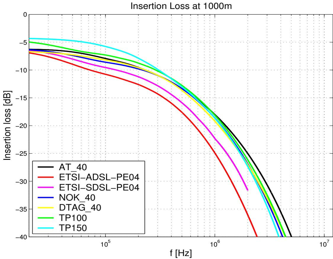
Figure 6: Comparing insertion loss for various 0.4mm cable models
