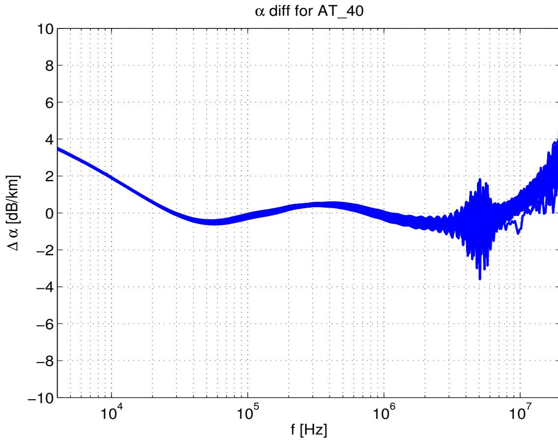
Figure 5: Comparing the difference between the insertion loss of the AT\_40 model (i.e., rounded) and the measured insertion loss
