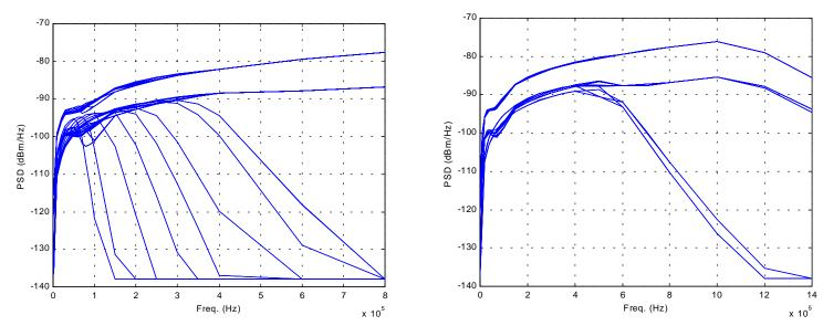
Piecewise Linear Noise PSD for symmetric and asymmetric PSDs on the LT side.
