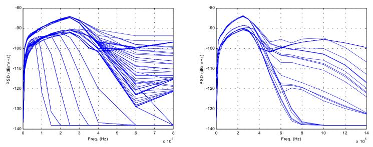
Piecewise Linear Noise PSD for symmetric and asymmetric PSDs on the NT side.
